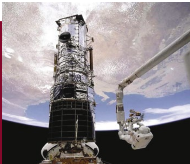
↑ During Hubble’s first servicing mission STS-61, astronaut Story Musgrave is anchored on the end of the Remote Manipulator System arm, ready to install protective covers on the magnetometers
