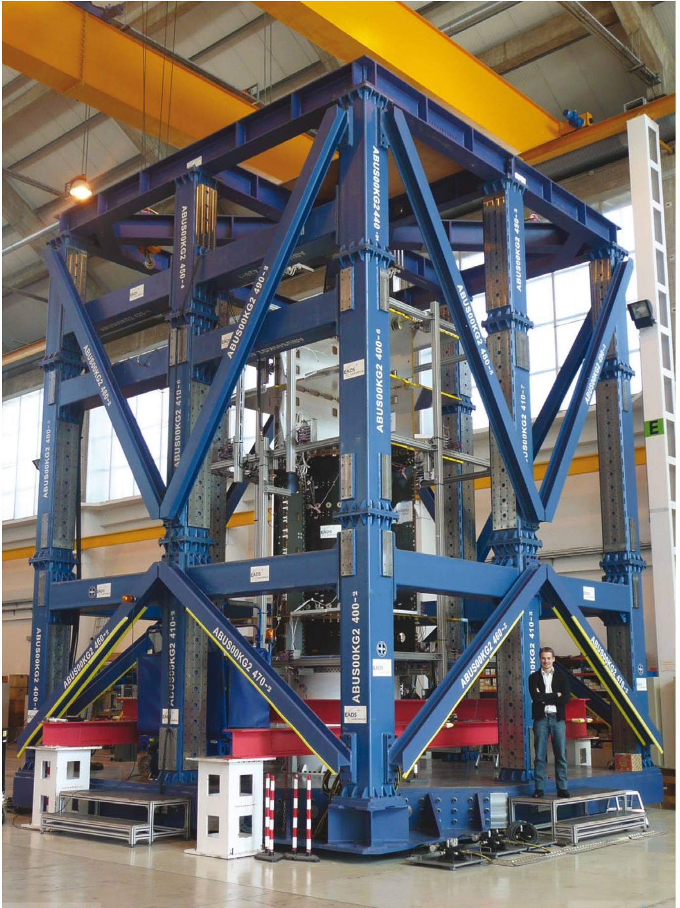
↑ Static qualification test stand (MMST) for the Alphaspace central tube and the primary structure at Inta (Spain)
