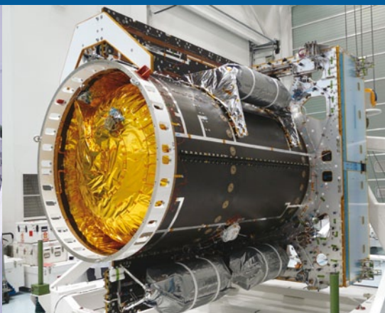
← Alphabus SM after mechanical integration in Thales Cannes, ready for transport to EADS Astrium Toulouse
