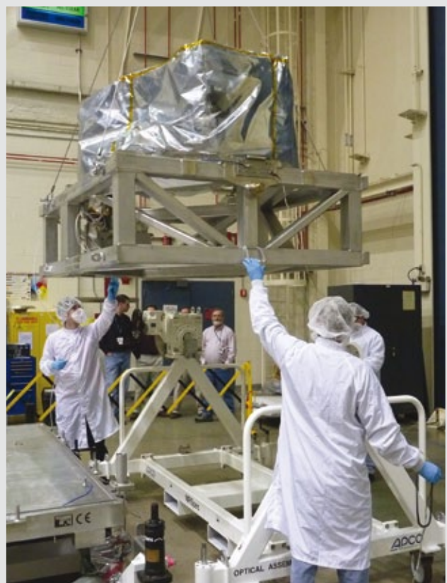
The JWST NIRSpec Engineering Model being unpacked at NASA Goddard Spaceflight Center
