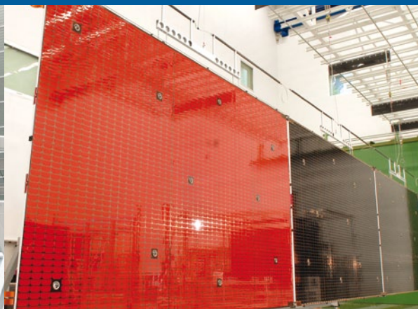
↑ Alphabus four-panel solar array wing, developed by EADS Astrium Ottobrunn (Germany), in deployed configuration
