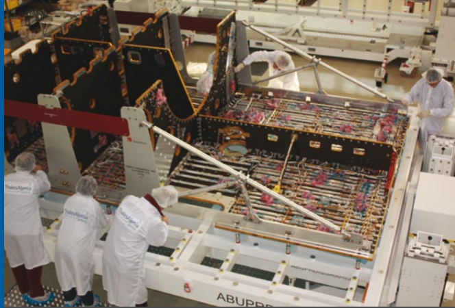
↑ The Half Repeater Module under assembly in Thales Alenia Space Turin (Italy)
