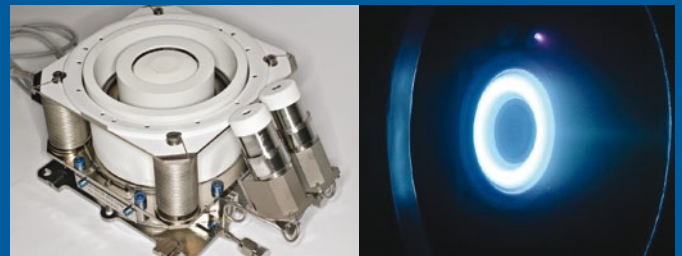
The PPS 1350-G plasma propulsion thruster developed by Snecma (France)
