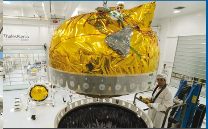
← Integration of one of the two main propellant tanks, developed by Man Technology Aerospace (Germany), into the Alphasat SM at Thales Alenia Space Cannes
