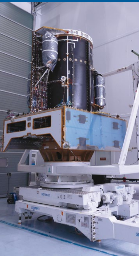
← Alphabus SM after mechanical integration in Thales Cannes, ready for transport to EADS Astrium Toulouse
