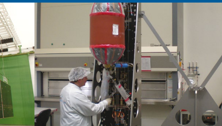
The Chemical Propulsion Module developed by Astrium Lampoldshausen (Germany)
