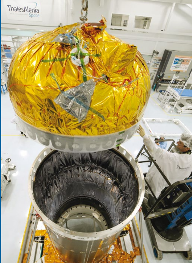
← Integration of one of the two main propellant tanks, developed by Man Technology Aerospace (Germany), into the Alphasat SM at Thales Alenia Space Cannes
