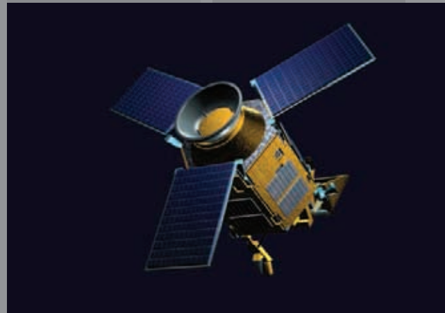
↑ To be launched in 2015, Sentinel-5 Precursor will be a satellite with a UV/IR spectrometer, developed to avoid a gap between Envisat and the launch of Sentinel-5 on a MetOp Second Generation satellite
