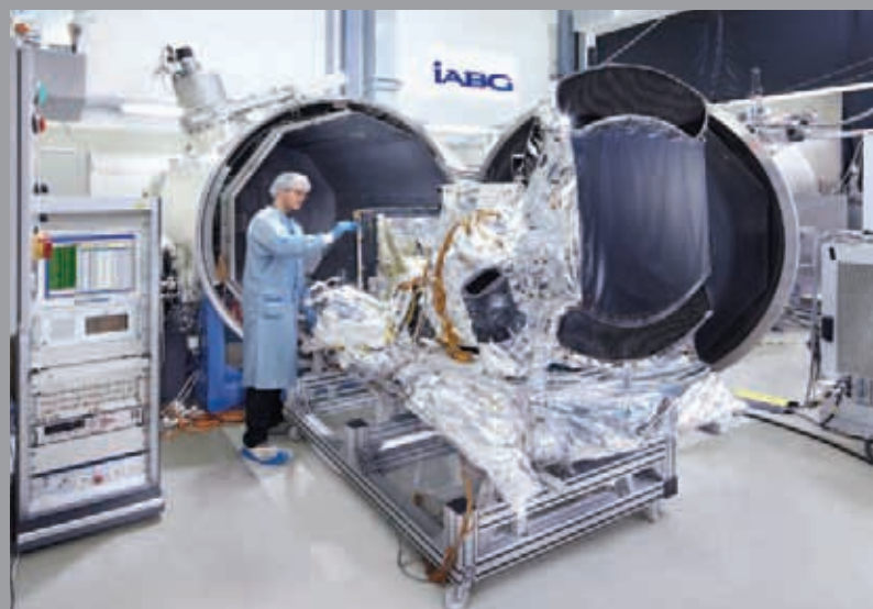
Sentinel-3 Sea and Land Surface Temperature Radiometer (SLSTR) STM entering the thermal chamber at IABG (IABG)
