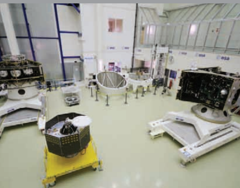
Structural Models of the BepiColombo MPO, MTM and MMO and Flight Model of MOSIF being prepared for mechanical tests at ESTEC
