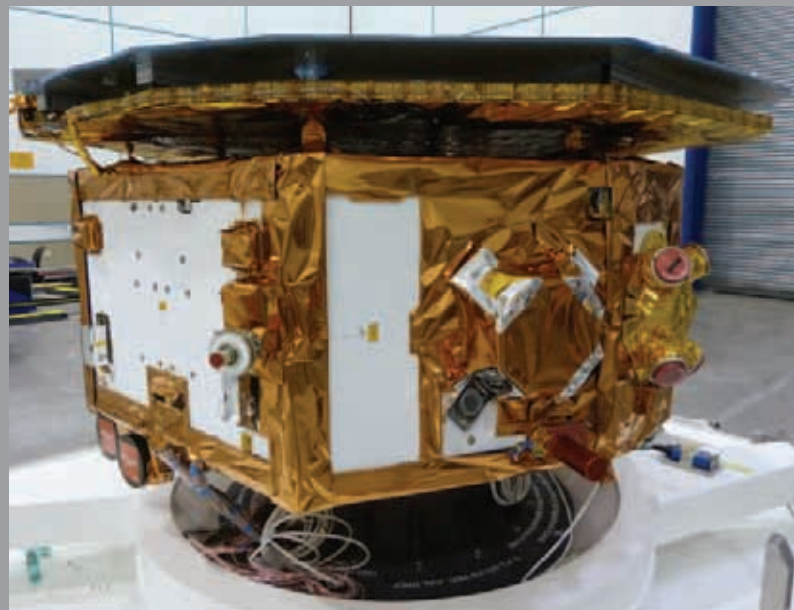
The LISA Pathfinder Science Module Flight Model after completion of the On-Station Thermal Vacuum Test at IABG, Ottobrunn (IABG/Astrium)
